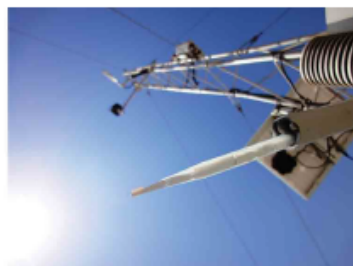
Figure 5. A minute "surface renewal" sensor (foreground in focus) for monitoring air parcels moving in the lower atmosphere. The sensor is mounted near the bottom of a meteorological mast with eddy covariance and energy balance equipment (background, out of focus).
